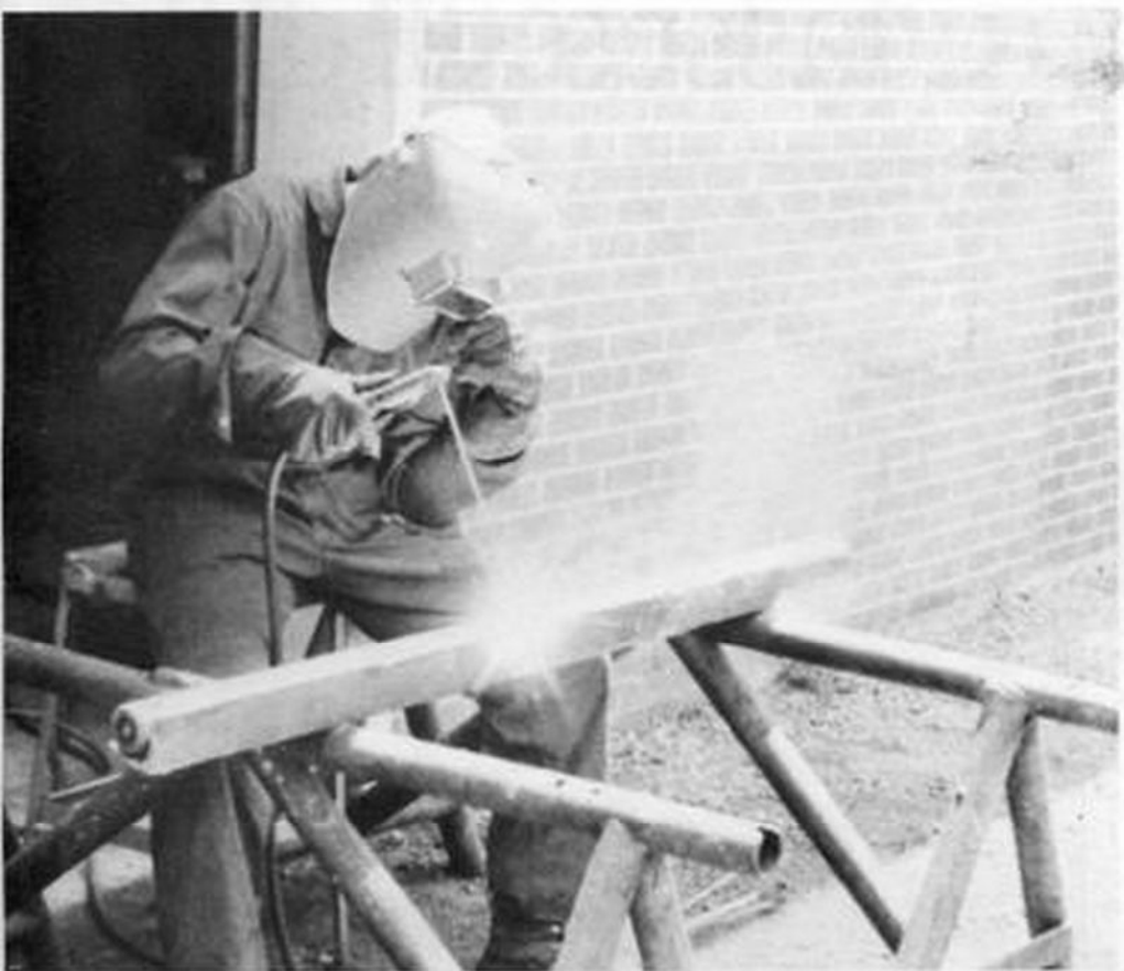
Mike Garber wears a welder's helmet for protection from welding flash and sparks.
